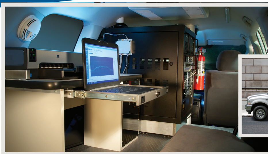
> Interior of Mobile station with with covert TCI Model 645 antenna mounted on a civilian vehicle.
